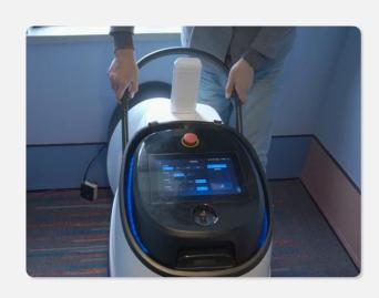
[Push robot away from charging pile] Switch robot to manual mode, push it away from charging pile.
