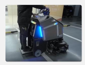
Drive robot to maintenance area, turn robot facing out and power it off. Please refer to "Operation Guide - driving operation" to drive robot.
