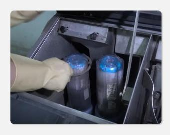
[Take filter bottles and cartridges off] Use wranch to loose the filter bottles anticlockwise, and remove the bottles and cartridges.
