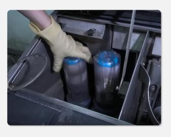
[Disassemble filter bottles]
