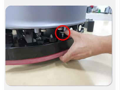
**5**.For install, insert the inner strip(the shorter one) first.
