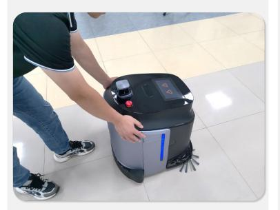
**3.**Open the side protection skirt first, press down and remove the shell of squeegee then move the lid left side to take it off.
