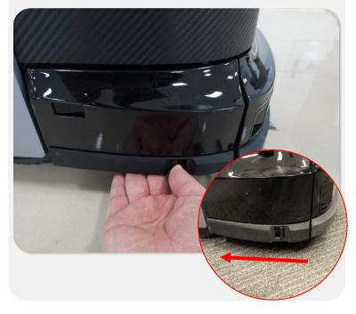
2.Grab the rubber boot and pull down to remove the side brush.Do not hold the bristles.
