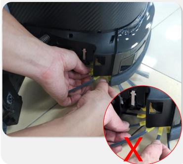
3.Clean side brush with wipes or replace it.Align the magnetic catch and push the side brush up to install it.
