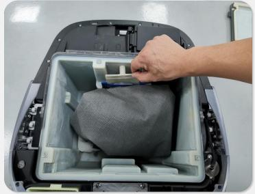
**6.**Pull the sealing strip out and empty the trash.
