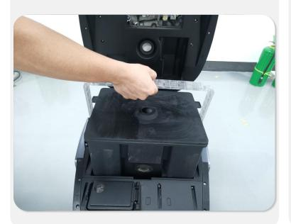
5. Remove the top cover of dust tank and take out dust bag .Notice: lift the white sheet up to seal the dust bag to prevent dust from spraying out.
