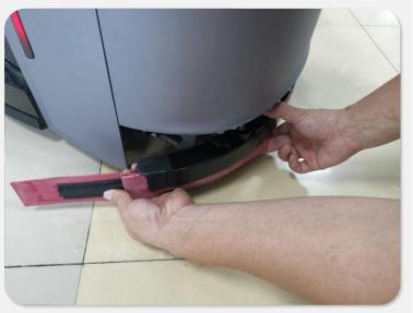
6.Install the shell back.Push the shell upward and cover the side strip.
